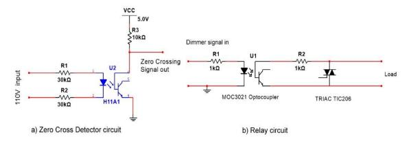
Figure 7. The zero-cross detector and solid-state relay
