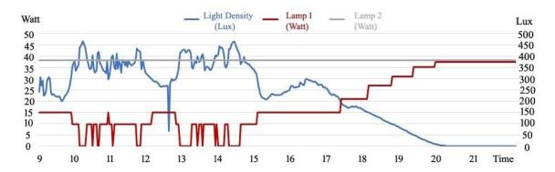
Figure 10. The light density and power consumption of the lamps
