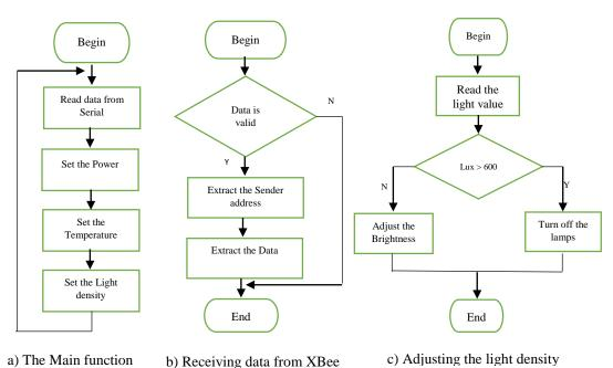
Figure 6. The flowchart of some functions in embedded software
