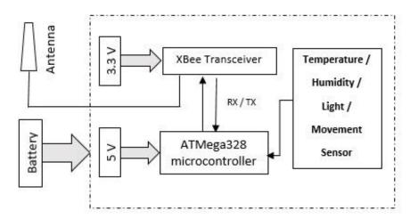
Figure 3. Block Diagram of a sensor node.
