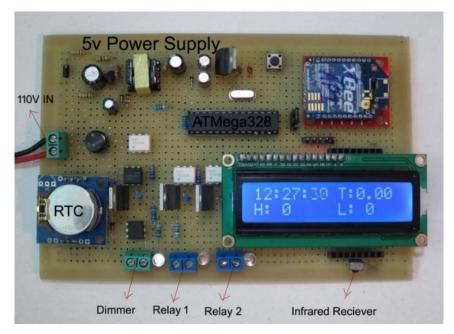
Figure 5. The prototype of the main controlling unit
